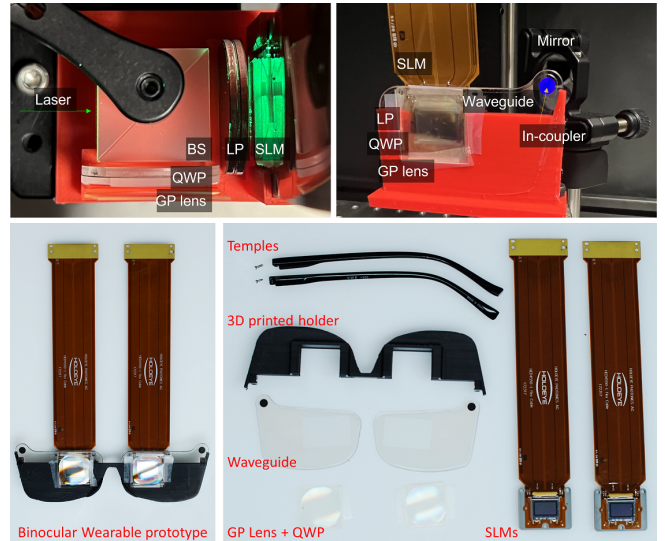
Fig. 5. Holographic Glasses prototype photos. Top-left: Optical bench prototype. Top-right: Monocular wearable prototype for testing. Bottom: Binocular wearable prototype used in Fig. 1.
