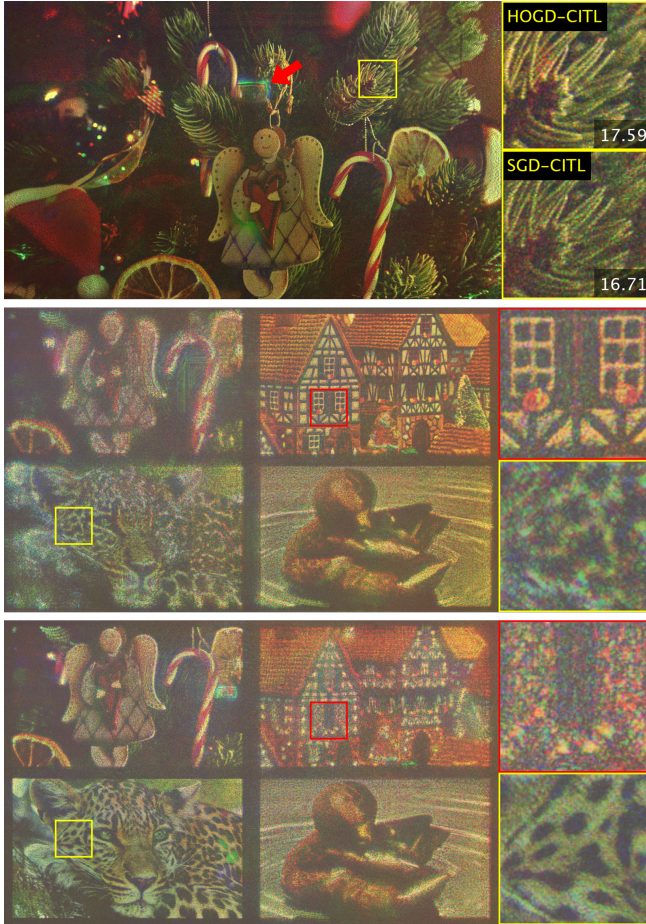
Fig. 8. Top : Captured 2D results from the optical bench prototype with the HOGD-CITL algorithm. The red arrow shows the artifact due to the GP lens loss. The close-up photo shows the comparison of HOGD-CITL and SGD-CITL. Center/Bottom : Captured multi-plane results from the optical bench prototype with 50 cm ( Center ) and 3 m ( bottom ) focus settings. The house and leopard scenes are located at a distance of 50 cm and 3 m, respectively.
