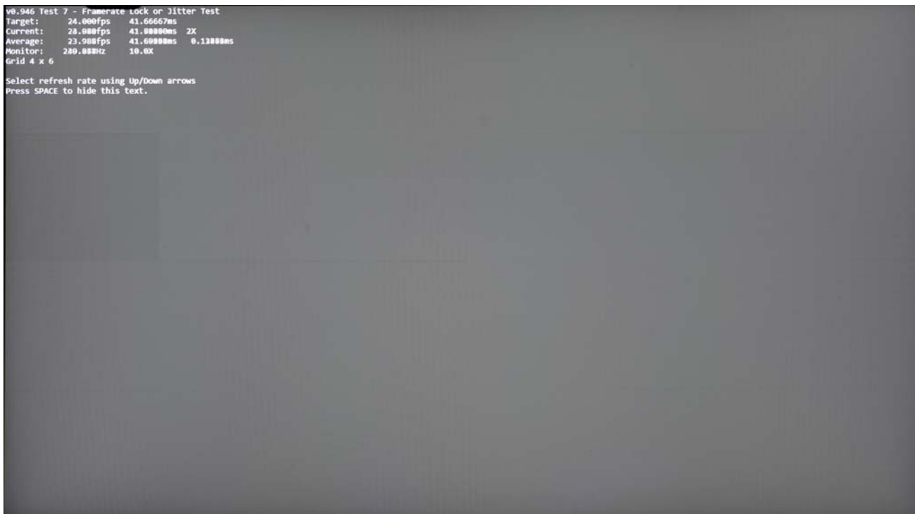
Figure 3-9: Example 24-Hz Test Results with Adaptive-Sync Operation Disabled (Informative)
