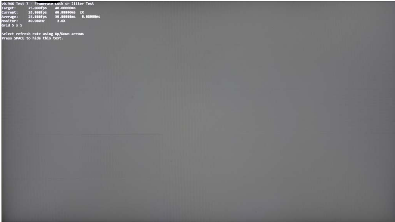
Figure 3-10: Example 25-Hz Test Results with Adaptive-Sync Operation Enabled (Informative)
