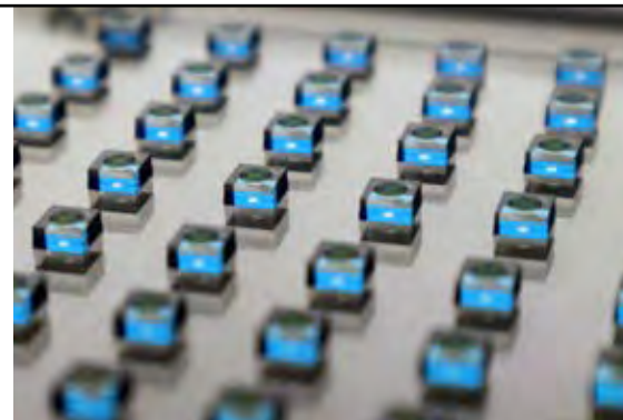
Close-up of NILT's "1M" metalens component, used inside the camera module being demonstrated at the company's exhibition booth this week in San Francisco. Photo: NIL Technology.
