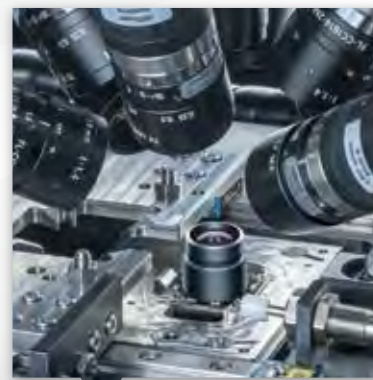
Alignment and testing of camera modules
