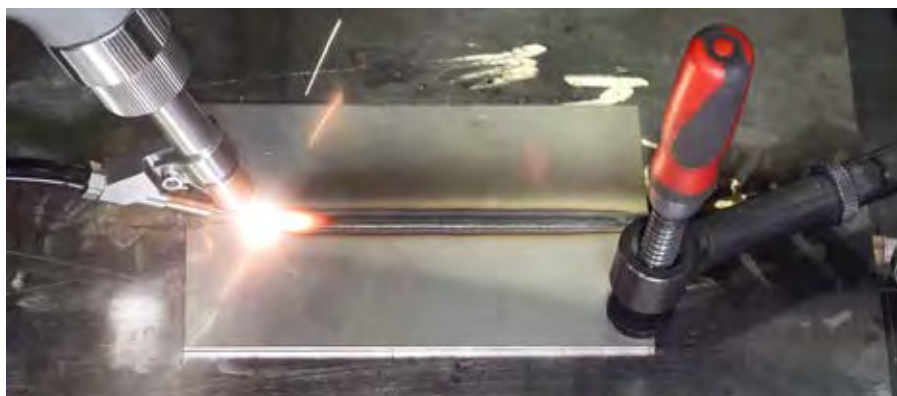
IPG Photonics' LightWELD system can achieve 100 percent weld consistency using preset programs. Credit: Courtesy of IPG Photonics
