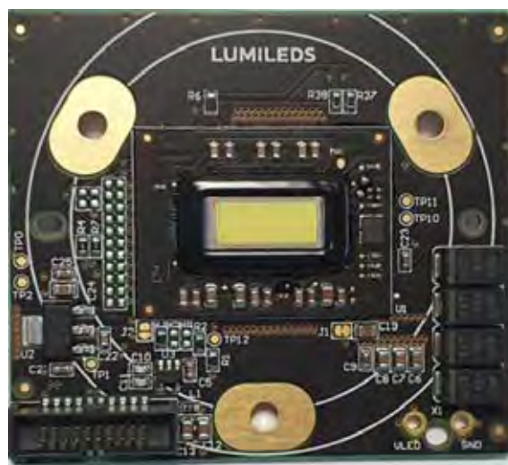
A Lumileds LED/CMOS hybrid digital light source. Credit: Courtesy of Lumileds.
