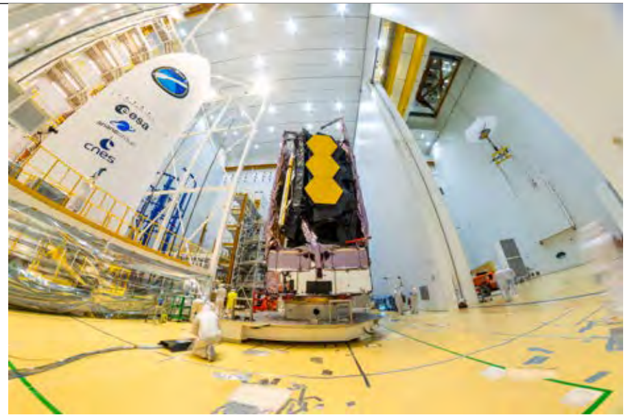
The James Webb Space Telescope, shown here two weeks ahead of launch as it was placed on top of the Ariane 5 rocket that carried it into space. Unfurling of the telescope’s sunshield and mirror optics represented two of the riskiest elements of the mission. Credit: ESA/M.Pedoussaut.
