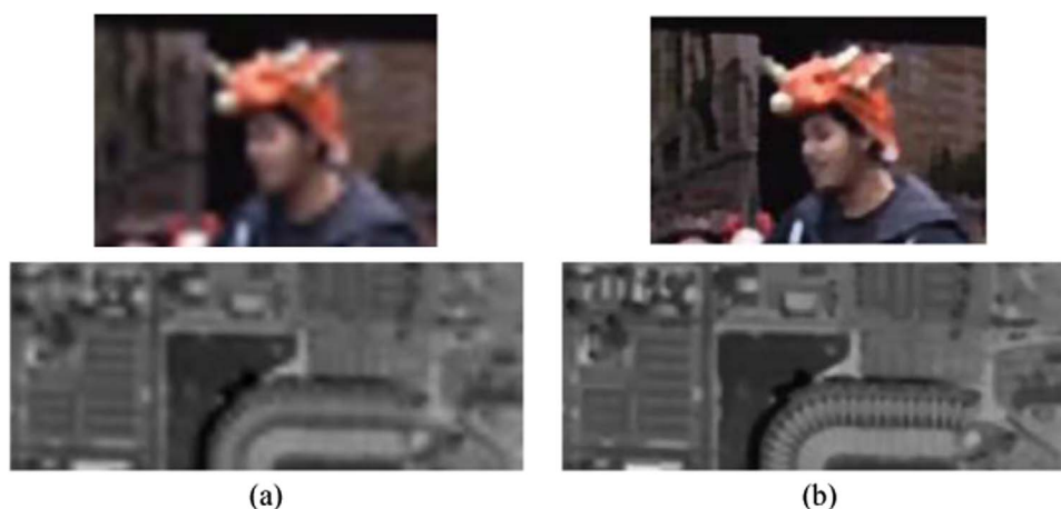
Fig. 11. The SR reconstruction of the Walk sequence (top row) [184] and a UAV surveillance sequence (bottom row) [66]: (a) indicates the reference LR frames, while (b) presents the corresponding reconstruction results.
