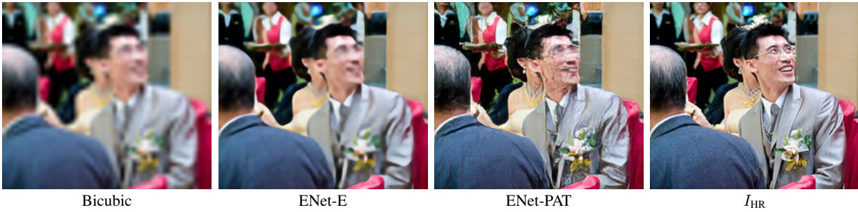
Figure 8. Failure case for ENet-PAT on an image from ImageNet at 4x super-resolution. While producing an overall sharper image than ENet-E, ENet-PAT fails to reproduce a realistically looking face, leading to a perceptually implausible result.
