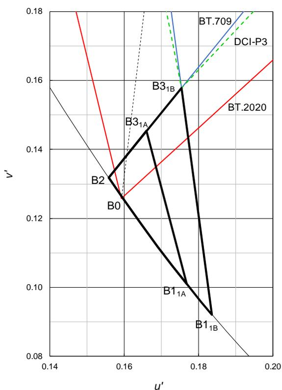
**Figure 7: CIE u'v' diagram of blue primary tolerances**
