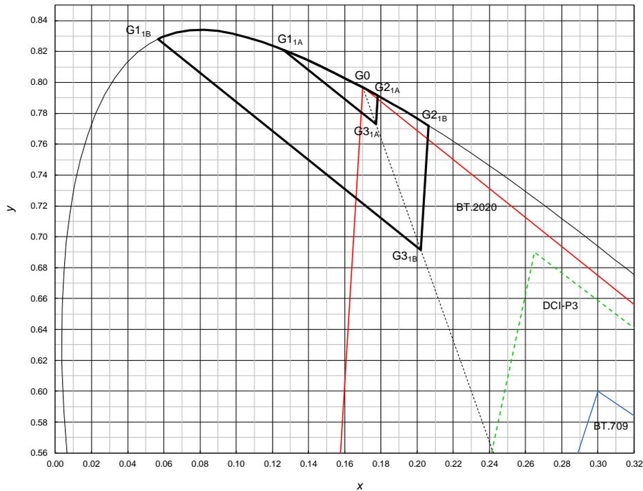
Figure 6: CIE xy diagram of green primary tolerances
