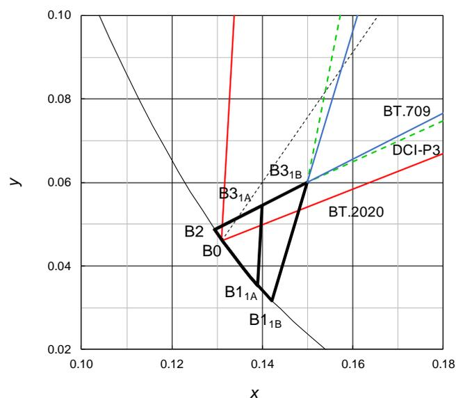
**Figure 8: CIE xy diagram of blue primary tolerances**
