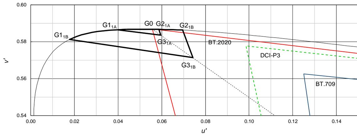
Figure 5: CIE u'v' diagram of green primary tolerances
