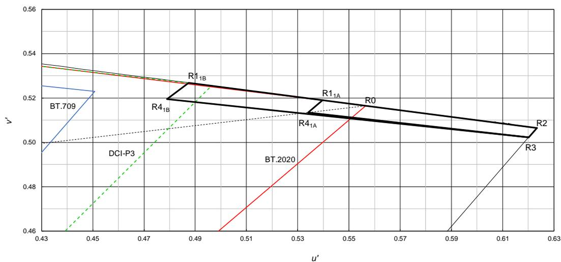
Figure 3: CIE  $u'v'$  diagram of red primary tolerances
