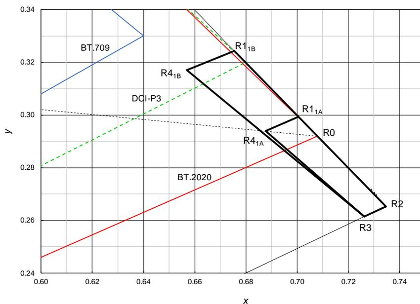
Figure 4: CIE  $xy$  diagram of red primary tolerances
