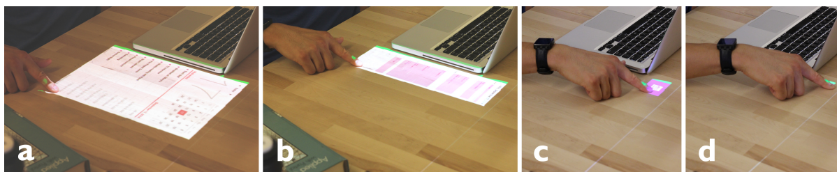
Figure 5. Resizing and closing . a: The user grabs the resize handle in the corner. b: Some interfaces can responsively alter their layout depending on their size; here, the calendar switches from week view to day view. c: Making the interface very small causes it to iconify. d: Shrinking the interface further will close it.
