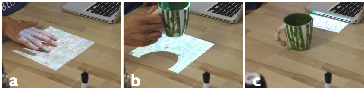
Figure 8. Evading and collapsing . a: An interface is positioned somewhere. b: The interface is occluded by an object. c: When the user moves his hands away, the interface evades the occlusion, and also collapses to fit available space.
