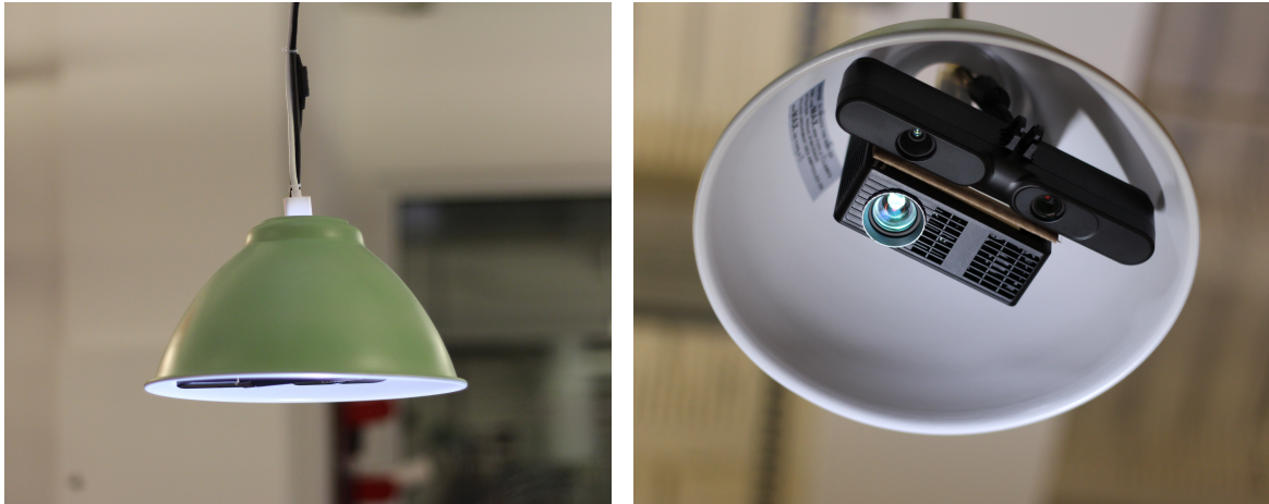
Figure 9. Our proof-of-concept projected augmented desk system fitted into a lampshade.
