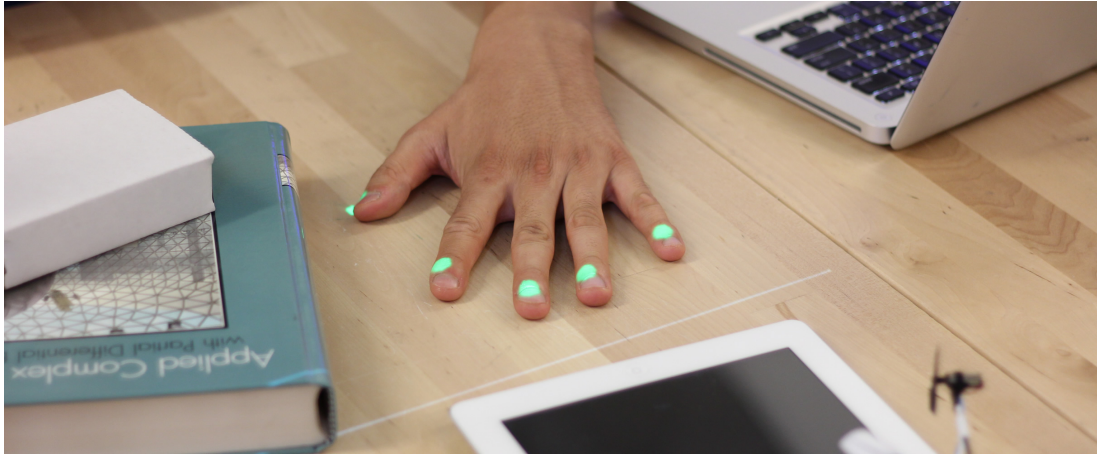
Figure 10. Our touch tracking algorithm can find fingertips even when the hand is flat against the surface.
