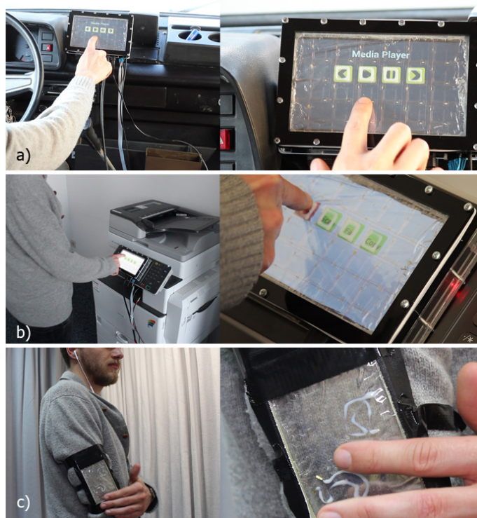
Figure 5. We built three additional demonstrators of GelTouch as a haptic a) car control panel, b) photocopier control, and c) transparent wearable armband.
