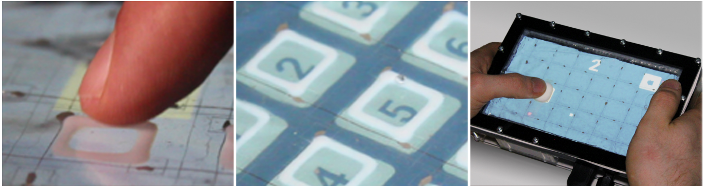
Figure 1. GelTouch is a thin gel-based layer that can selectively transition between soft and stiff (up to 25 times stiffer) within seconds to provide multi-touch tactile feedback. Activated areas can be changed continuously and dynamically. We show that GelTouch can be applied to touch screens and that screen elements such as buttons, sliders and virtual thumbsticks can be augmented with tactile guides. This can enable eyes-free interaction (e.g., typing) and improve the user experience of tablets, control panels of cars and appliances, and wearables.
